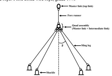
**Figure E-2** Four legged Wire Rope Lifting Sling with Fore runner
