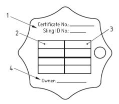
Figure 8-2 Example of identification tag for a chain sling – Back of identification tag
