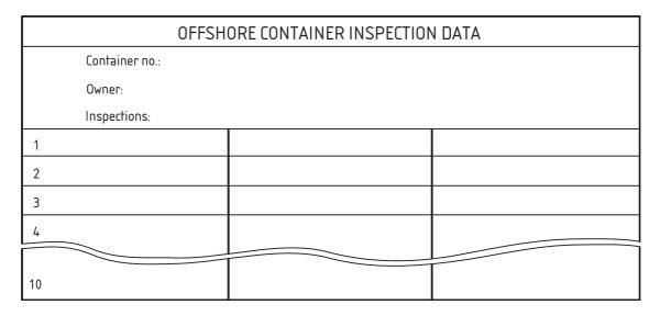
NOTE The information required for the inspection plate may be combined with the Offshore Container Data Plate (see EN 12079 - 1).
